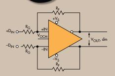
I. Some differential voltage feedback amplifiers include an additional  $V_{\rm OCM}$  input that allows the common-mode voltage of the output signal to be shifted.
