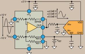
2. A level-translating driver, optimized for specific ADCs, provides a convenient way to accurately match the wide voltage output of sensors excited by  $\pm 10$  V (common in industrial applications) to a single-ended ADC input with a more restricted voltage range.
